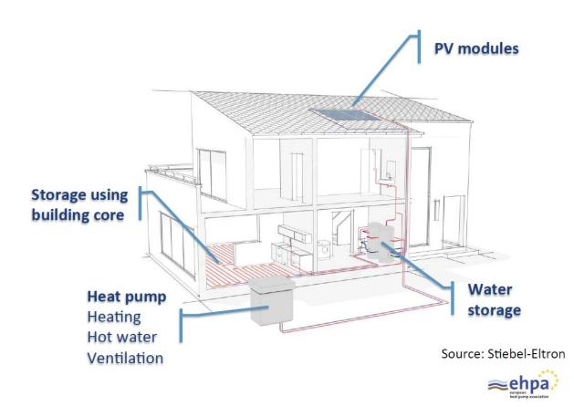
Figure 3 – Typical combination of heat pumps and PV in a residential building
