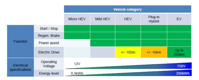
Each vehicle type places a different set of demands on the installed battery or batteries, according to the e-mobility services that must be provided. A portfolio of different battery technologies is required to fulfil these demands.
